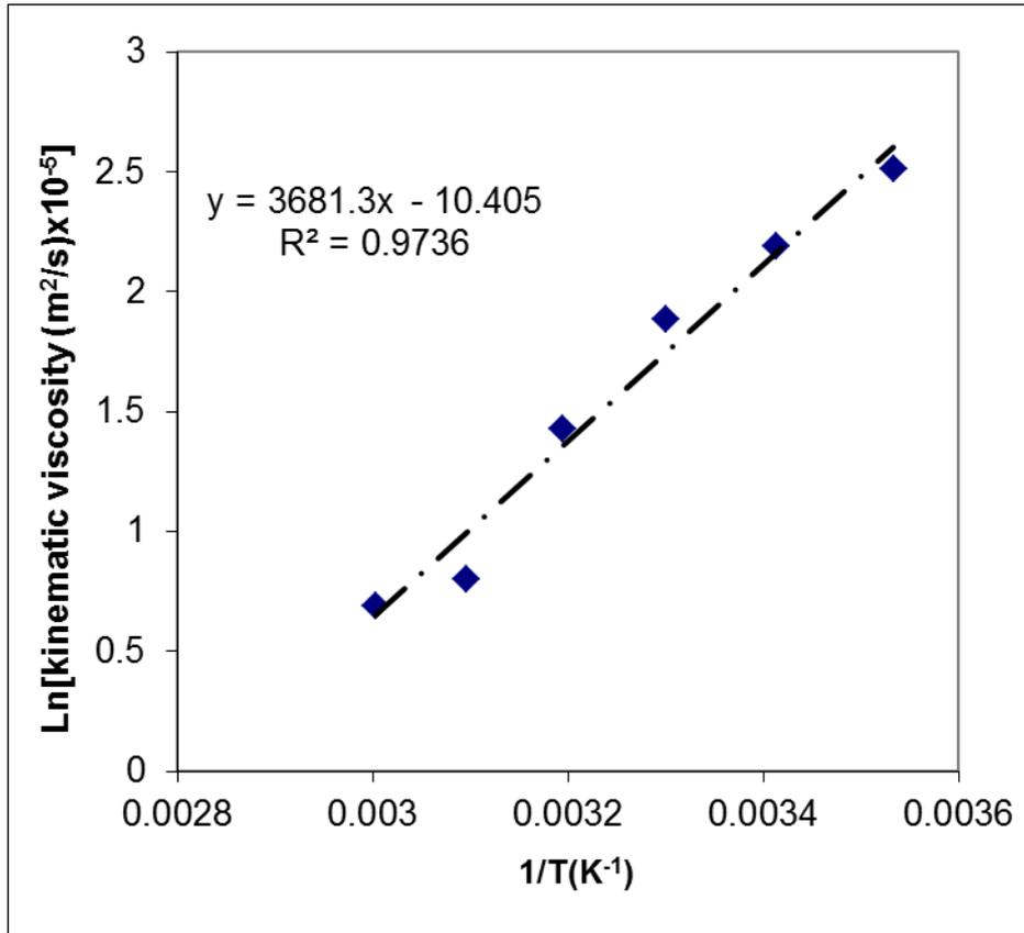
Figure 4: Dependence of Ln(viscosity) versus 1/T of avocado oil.
