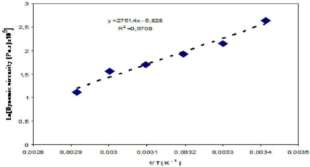
Figure 6: Dependence of Ln(viscosity) versus 1/T of rapeseed oil.
