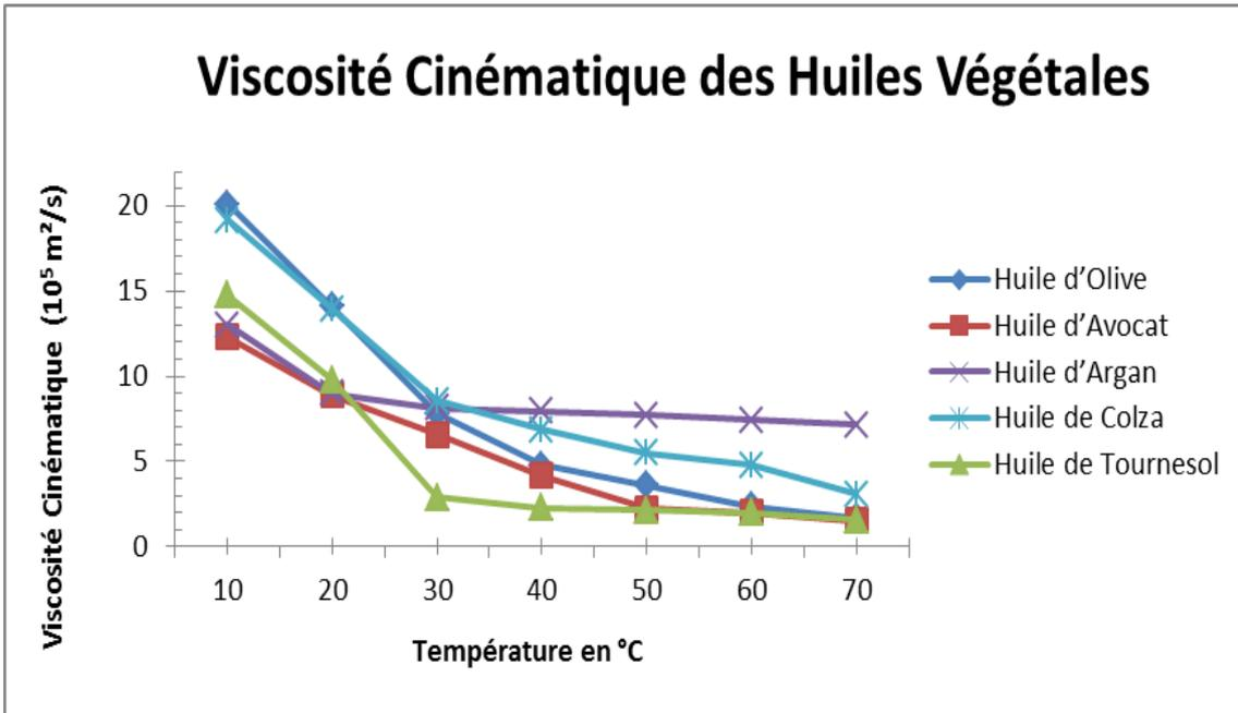
Figure 2: Kinematic viscosity of the different vegetable oils
